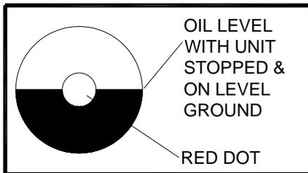
3. Change the crankcase oil after the **first 50 hours** of operation. Drain and refill the crankcase oil **every 500 hours** thereafter.
